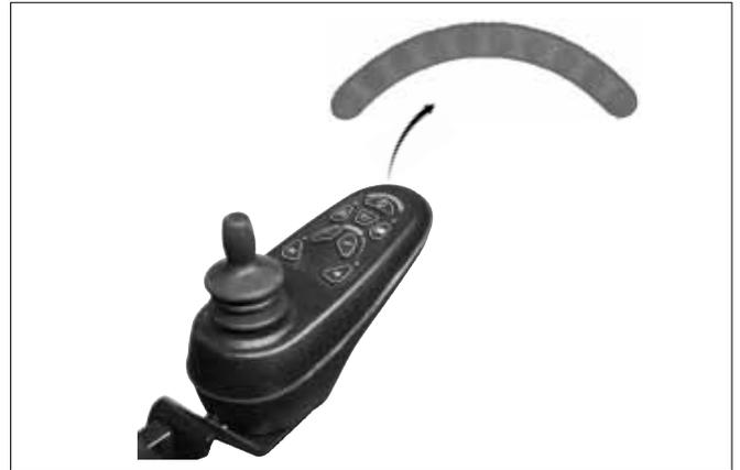
**5 segments blinks:** The electrical connection to the right motor is defective (short-circuit). Check the motor connection cable, motor cable plug and motor.
